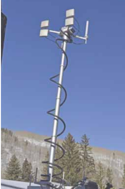
A deployable cell on wheels (COW) provided coverage for the race venue.
